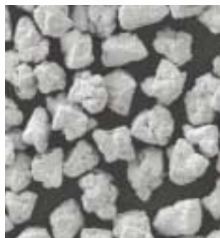
SPR Cu50 Diamond Copper coated Coating level 50 wt %
