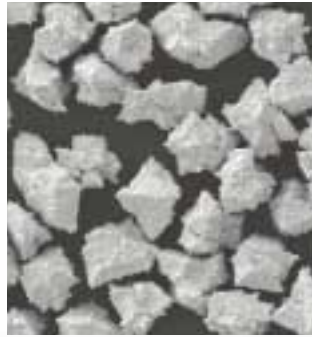
SPR N Diamond Nickel based alloy coating Coating level 56 wt %
