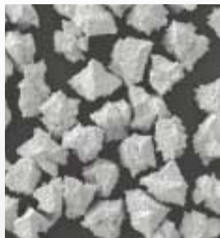
SPR N 30 Diamond Nickel based alloy coating Coating level 30 wt %
