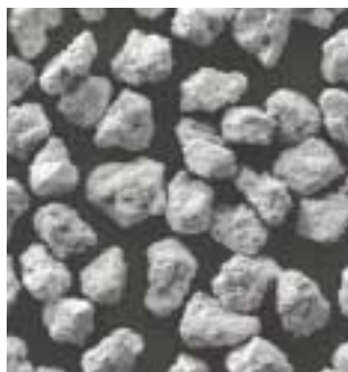
RVG 810 D Diamond Copper based alloy coating Coating level 50 wt %
